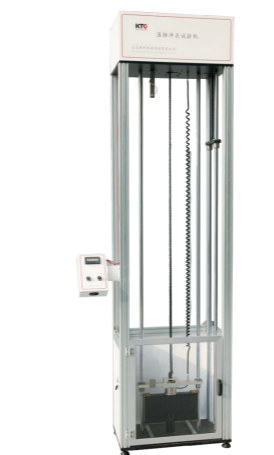
낙하충격시험기 Falling Weight Impact Testing Machine
