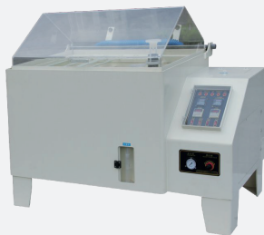
염수분무부식시험기 Salt Spray Corrosion Testing Machine
