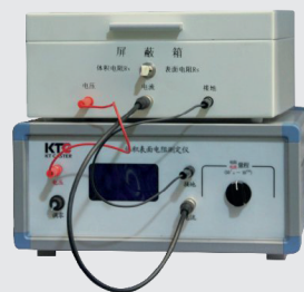
저항시험기 Resistance Measuring Instrument
