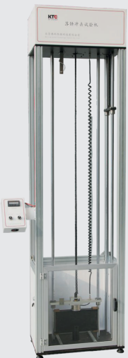
낙하충격시험기 Falling Weight Impact Testing Machine
